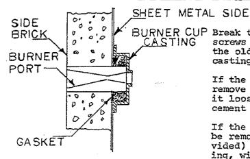
BURNER CUP Break the union in the piping. Loosen the CASTING screws and remove the cup casting. Remove the old gasket and any cement from the cup casting.
