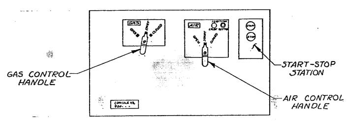
NOTE: IF FURNACE HAS BEEN IN OPERATION, ALWAYS WAIT AT LEAST 5 MINUTES BETWEEN SHUT DOWN AND STARTING UP OF THE FURNACE.
