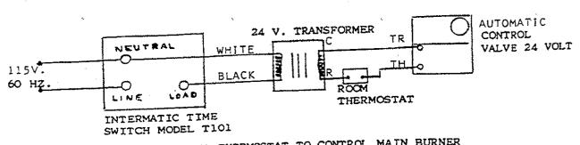
USING TIME SWITCH AND THERMOSTAT TO CONTROL MAIN BURNER
